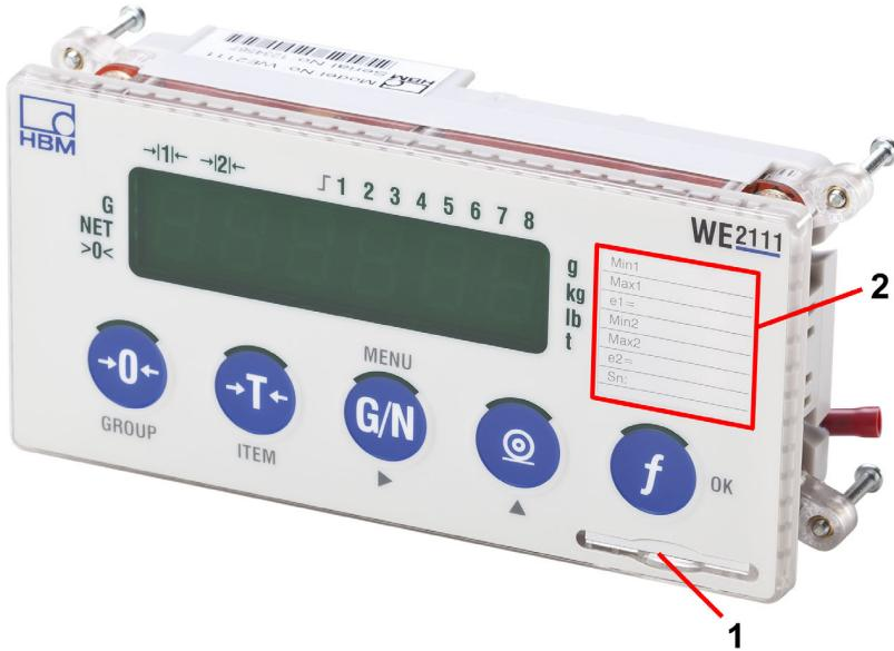
Fig. 2: Insert plug-in card in position 1. The card will then be displayed in the window at position 2. Then seal the place of position 1 with a calibration label.
